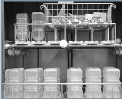
Compact cabinets for washing and/or drying feeding bottles, cans and other utensils such as buckets, pans, etc.
