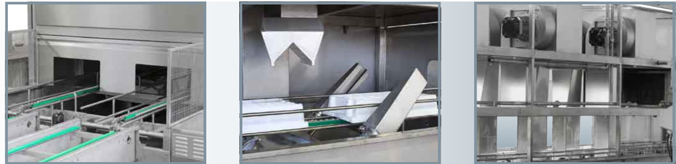
Modular tunnels for blowing and/or drying boxes, trays, pallets, "palot" containers, etc., that can be coupled to the washing tunnels
