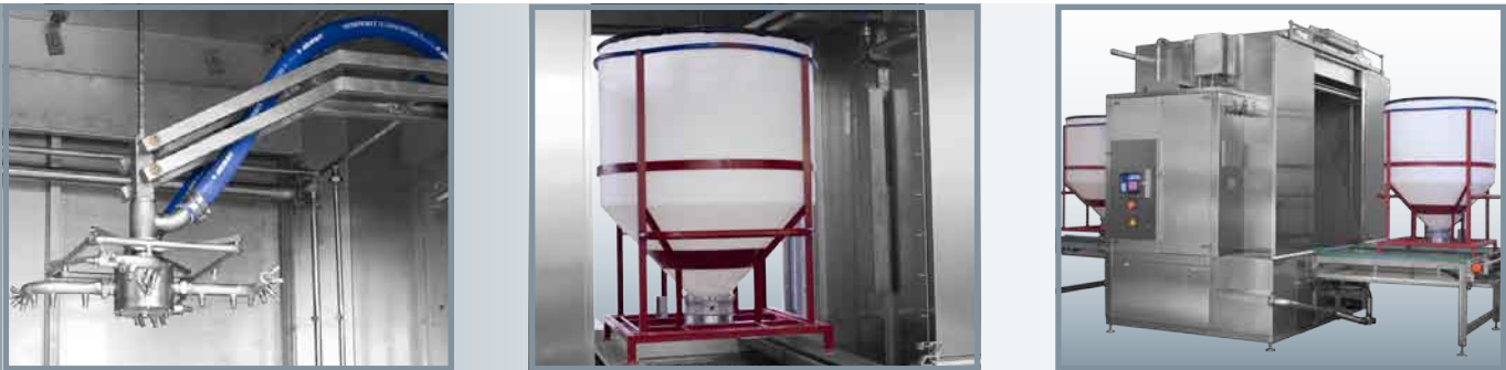
High-performance cabinet for washing tanks
