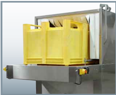
Compact tunnels for high-power washing of “palot” containers, adaptable for washing boxes
