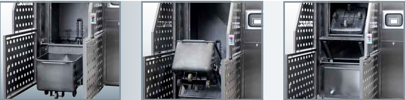
High-performance cabinet for washing meat trolleys
